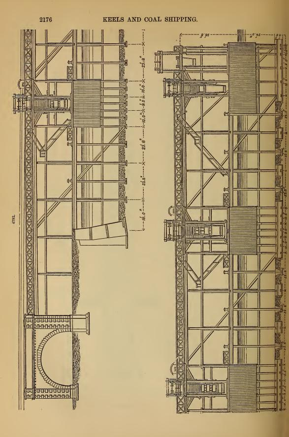
lengthened experiments were made on the ground above, where a complete plan of the proposed arrangement, for one spout, was laid down; and on it, wagons of all classes in use were tried, under different states of weather and circumstances. The result was that the inclinations adopted, which are much steeper than theory would give, were found to be necessary.
